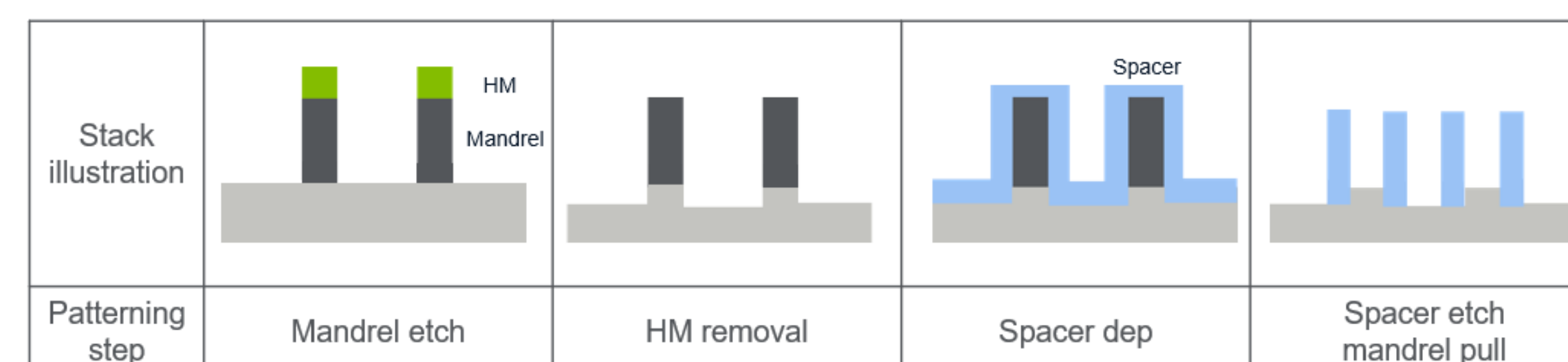
Fig. 2 SADP stack and process flow illustration.
