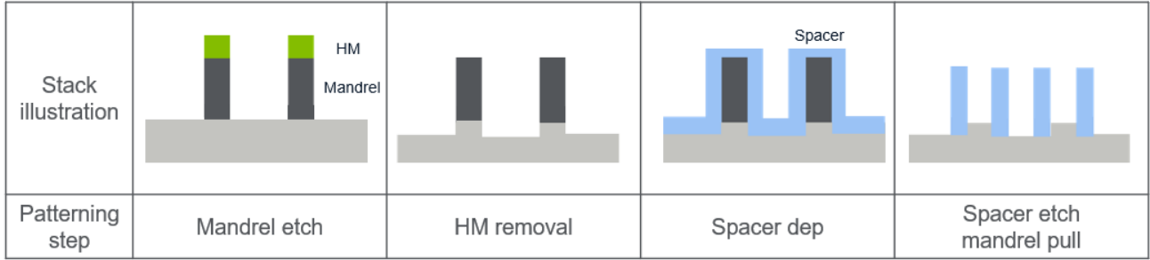
Fig. 2 SADP stack and process flow illustration.
